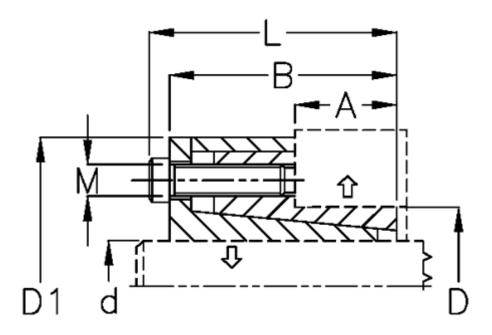
A mm = 37 B mm = 60.0 D1 mm = 96.5 d H8 mm = 30 D mm = 72 F kN torque = 105 L mm = 68.0 M mm = 8 P N/mm2 surface pressure on shaft/hub = 99
